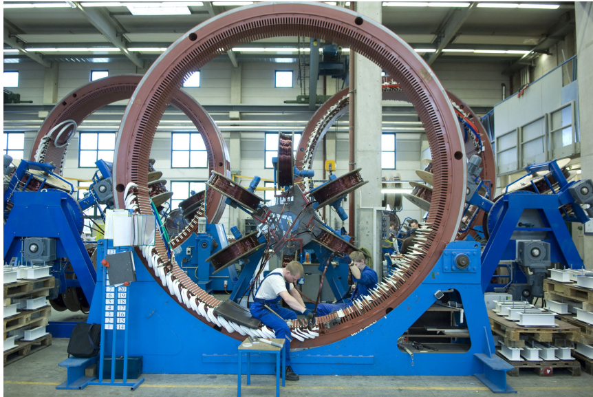
Figure 2: Manual insertion of the copper windings into the generator stator. (Courtesy of Enercon.)
