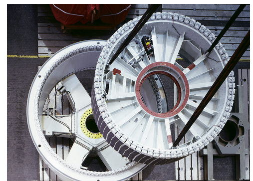
Figure 5: The huge magnetic rotor is lowered into the stator coil. Compare with Figure 4 to see how large the rotor is. (Courtesy of Enercon.)
