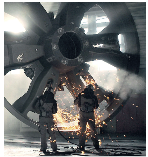
Figure 4: This picture shows the size of the generator rotor. The workers are 2 metres tall. (Courtesy of Enercon.)
